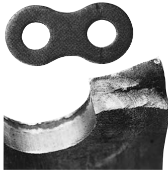
② Fatigue fracture By repeatedly applying a load past its fatigue limit (fatigue strength), the fatigue will start at holes and then cause sudden chain breakage.
