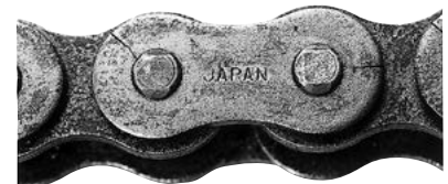
Fig. 32 Hydrogen embrittlement cracking
