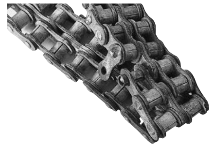
Fig. 31 Corrosion of stainless steel roller chain
