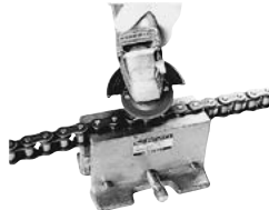
Fig. 2 Grinding the pin ends
