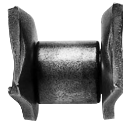
③ Offset link plate fatigue Offset link plates are bent at the center, and the resulting concentration of stress at the bend can cause a fatigue break. Avoid using offset links in high-stress applications.
